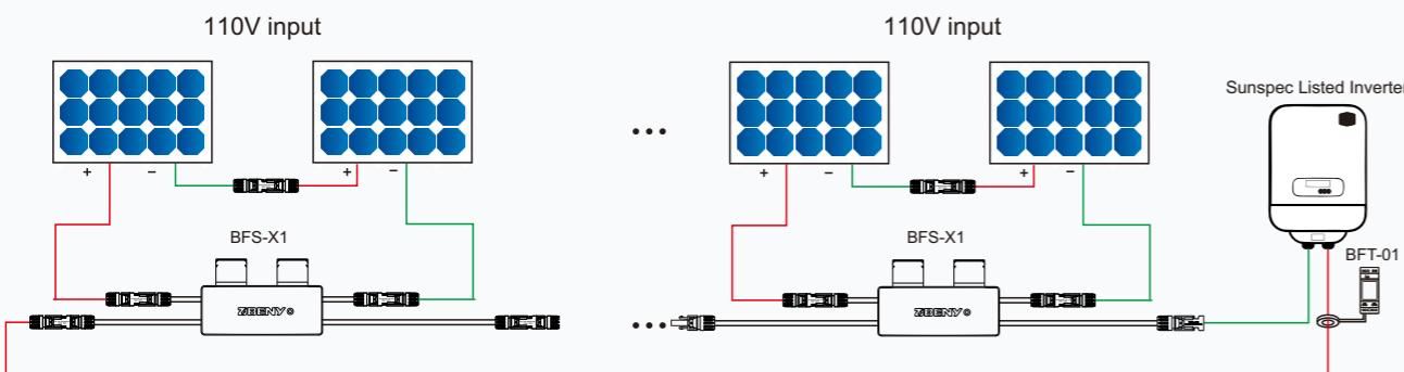
Each BFS-21/BFS-22/BFS-X1 device can hold solar modules output max: 1500V total, the modules connect in series as solar string goes to inverter as PV system designing. The connection of BFS-21/BFS-22/BFS-X1 RSD and Rapid Shutdown Monitoring Device is via communication cable.
