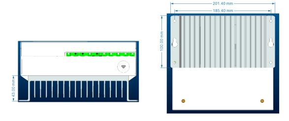
Choose any set of mounting holes, and install the controller vertically on the wall with expansion screws.
