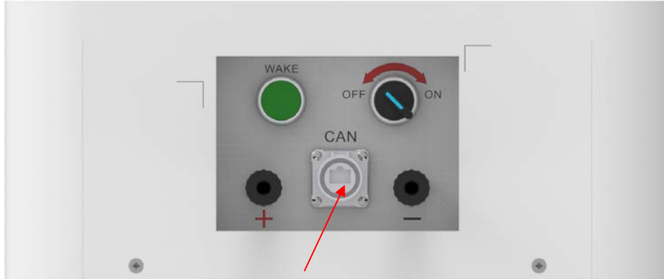
Connect to inverter RJ45 CAN communication port
